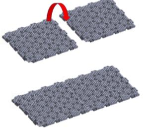
Continue snapping panels together until reaching the opposite side, then start on the next row. Panels can be staggered as well. Be sure to leave ~½" gap between fixed objects such as curbs and posts. For larger installations, a stringline can help with staging the panels into rows, as well as keeping the rows straight.
